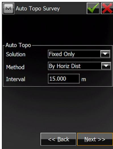
Auto Topo options, for automatic point collection by time or by distance. The interval and Method can be defined as required.
