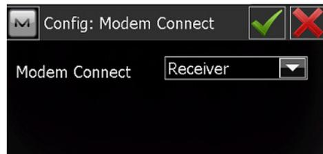
The Modem Connect should be set to Receiver in this case if a field controller is used which does not
