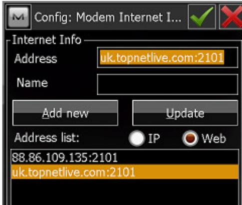
Either method works in MagNET Field although the host name is the preferred method of connecting from a user point of view. It reduces the potential need to change IP addresses should any server issues arise.
