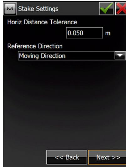
The default is 50mm for setting out, this can be defined by the user as can the reference direction.
