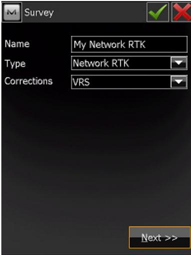
Now we start with the editable options in the configuration. The configuration name can be changed if required.
