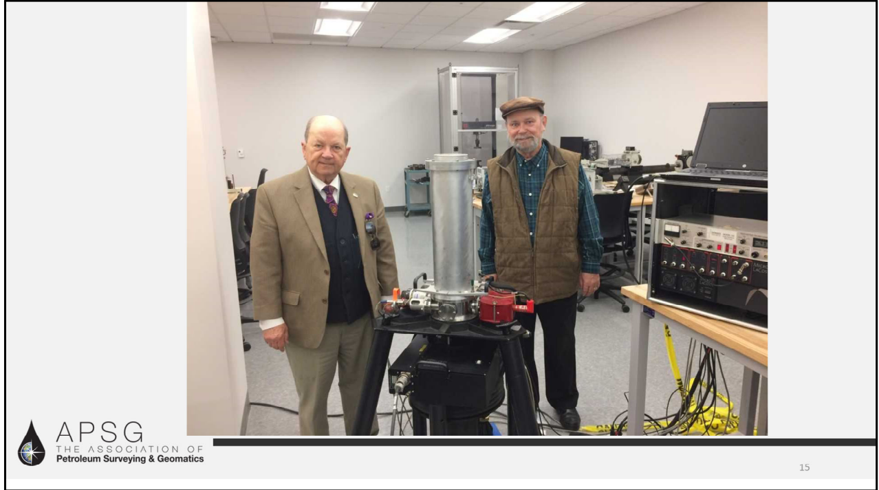
NGA's FG5 Absolute Gravity Meter. (Observing time about 1 day – only indoors.)
