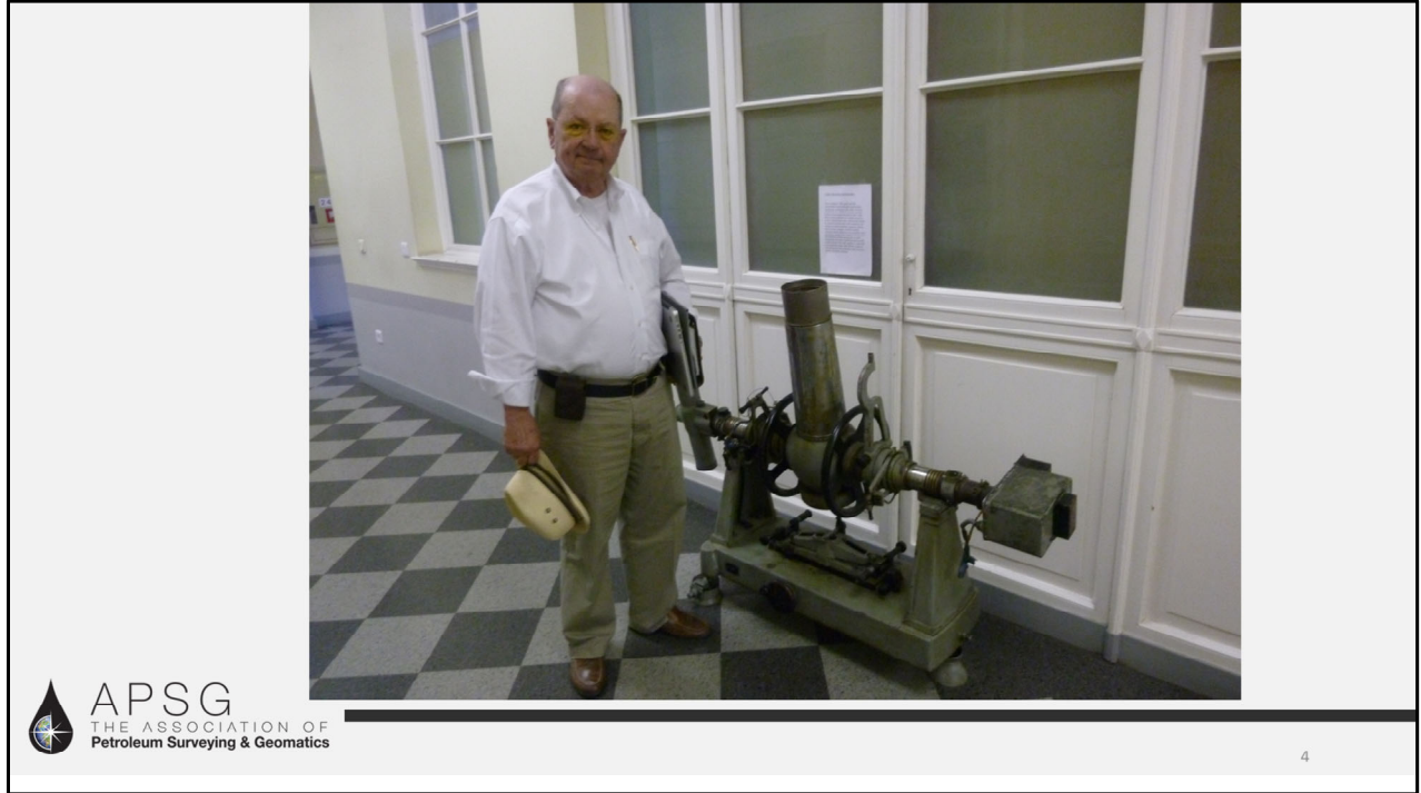
Broken elbow astronomical theodolite at the University of Latvia. Used as a Transit Telescope, (c.a. 1860s)
