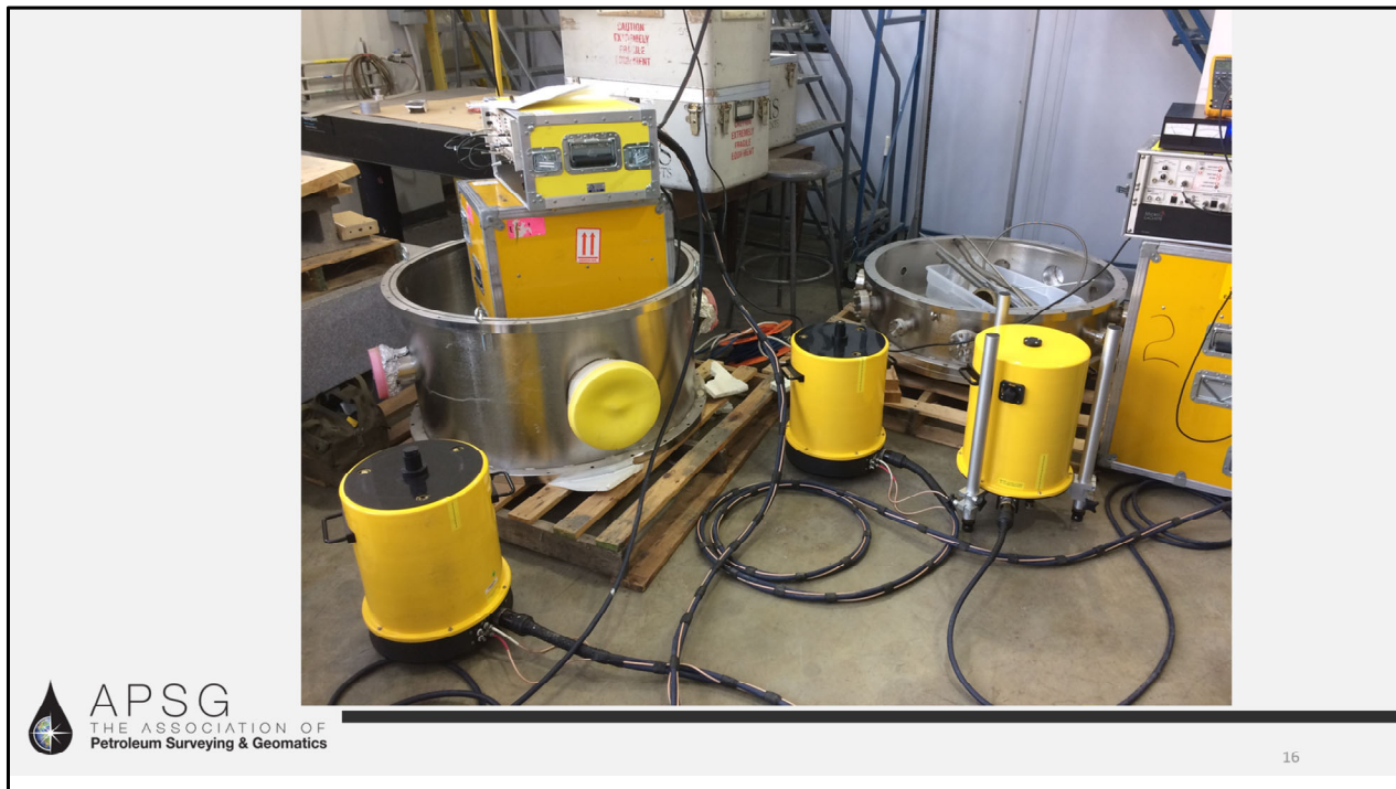
NGA's Absolute Gravity Meters (A-10) used for observations outdoors. (Observing time under 1 hour.)
