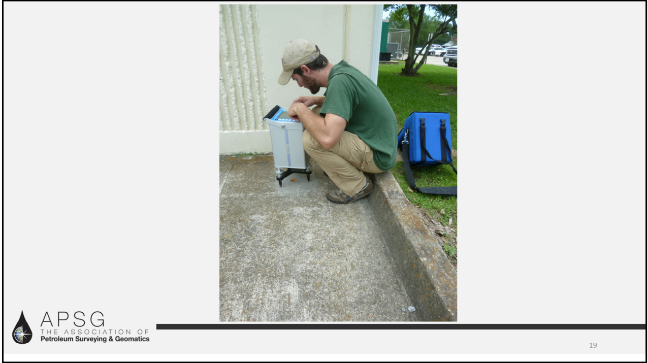
Relative Gravity observation with a Scintrex CG5.
