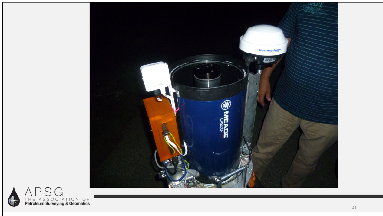
Latvian Digital Zenith Camera (DZC). (This is serial #2 – LSU instrument will be #3.)
