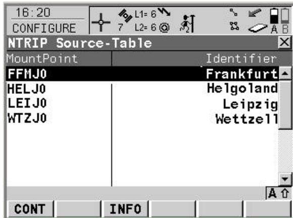
A Mountpoint can be selected with **F1(CONT)**. To view information about a particular Mountpoint, press **F3(INFO)** to access the **CONFIGURE Mountpoint** panel.
