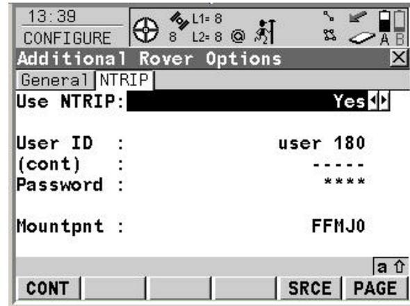
In order to access and receive RTK data from the NTRIP Caster a **User Id** and **Password** needs to be entered. If necessary, contact your NTRIP administrator to obtain a User ID and password.
