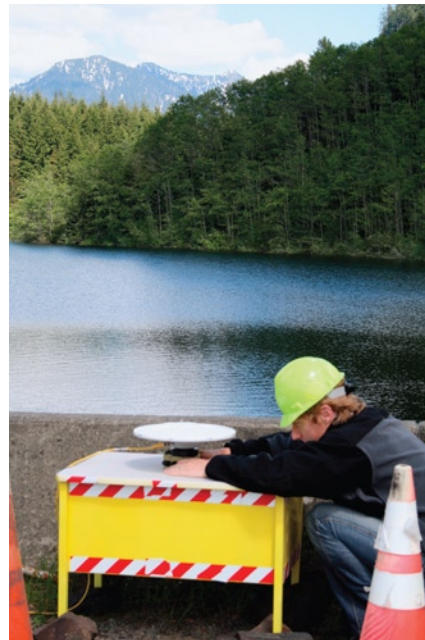
Figure 3 Controlled movement tests; displacements marked on a graph sheet on a level table.
