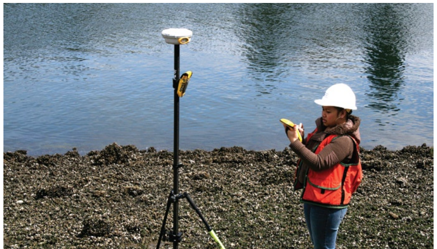
Figure 3 This handheld unit has its own built-in receiver, but the user has chosen the option of connecting to a more powerful dual-frequency receiver. In this example of shoreline work, better vertical was needed than the mapping unit could provide on its own.
