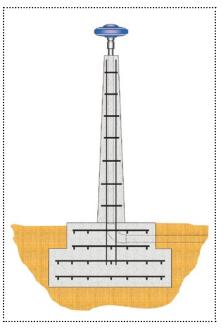
One of many similar variations. this seeks to provide a heavy-stable base for a pillar. Reinforced concrete provides mass, with a broad base. Some have experimented with low, squat pyramids, but those can present a multi-path hazard; the pillar reduces this. Like other good designs, the antenna mount should be 1.5m above the ground to reduce multi-path hazards.
