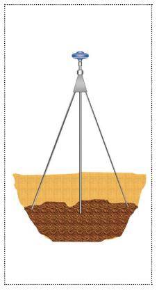
This can be used when the depth to bedrock or other stable surface is less than 10 feet. The stability of a tripod (though most constructed have 4 angled legs plus one vertical under the antenna) is paired with narrow members (to reduce multipath hazards). This is very popular with the scientific community, okay by both Unavco and NGS standards.
