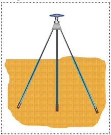
Another tripod, "quad-pod", or "quintpod" style monument, this one is used where the soil and sub-surface conditions may be less stable. The legs may be drilled up to 40 feet and only cemented into place at the very bottom; the balance of the hole around each leg is filled with an insulating material that will not place drag on the legs in the event of shallow strata shifting or sub-surface expansioncontraction.
