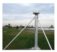
There are often old foundations or pads available (decommissioned communications sites or old cold-war-era antenna farms often have lots of stable pads), or there may be ground-level concrete utility vaults on which to attach a brace pole. This same type of mount is often used at the corners of load-bearing walls or parapet walls on very stable buildings. How high can one go on a building? There are too many variables to consider, therefore testing is often the best practice.
