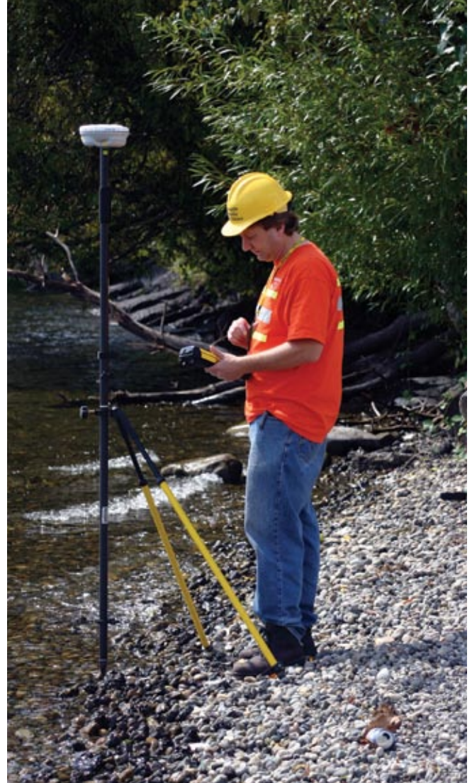
Equipment manufacturers have introduced network-ready gear that is interoperable with the multiple flavor real-time networks. The two brands pictured are being used at the same time, utilizing the same RTN, for an emergency drainage investigation. RTN enabled rapid mobilization and feedback to the investigators.
