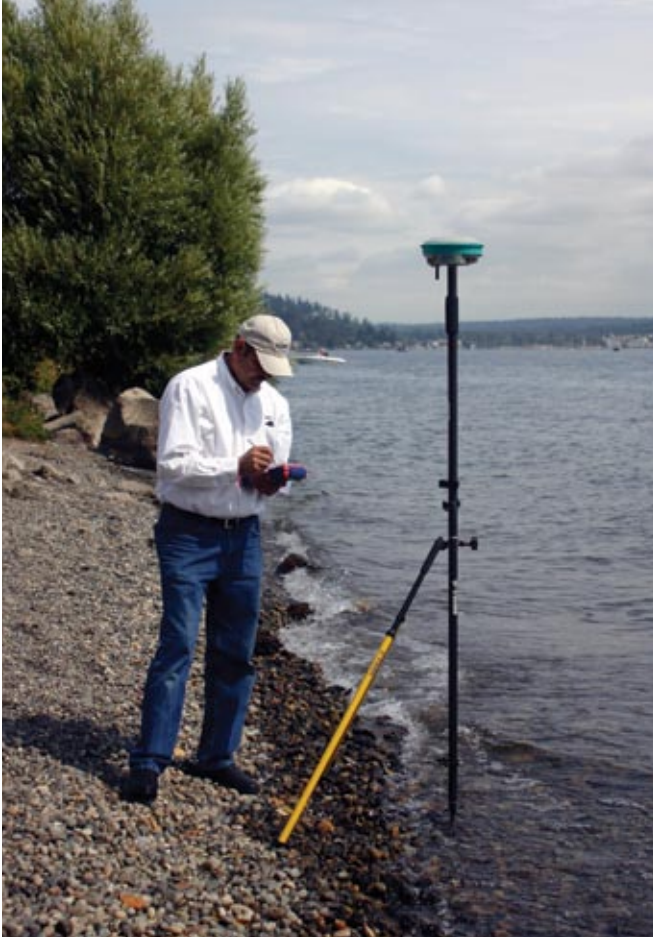
Equipment manufacturers have introduced network-ready gear that is interoperable with the multiple flavor real-time networks. The two brands pictured are being used at the same time, utilizing the same RTN, for an emergency drainage investigation. RTN enabled rapid mobilization and feedback to the investigators.
