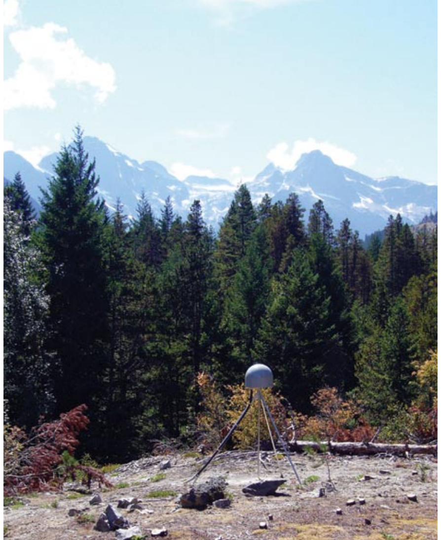
Multi-purpose CORS at Ross Dam in the North Cascade mountain — UNAVCO Plate Boundary Observatory and Seattle City Light — joint venture for geophysical studies, dam operations, surveying, mapping, and monitoring.
