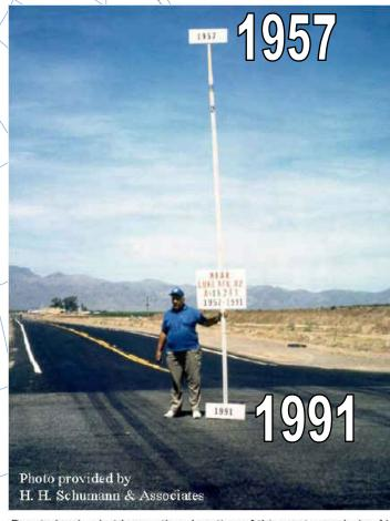
Due to land subsidence, the elevation of this spot near Luke Air Force Base in Maricopa County has dropped by more than 18 /feet over a 34-year period. Knowledge of subsidence areas is a fundamental requirement for planning infrastructure such as pipelines, canals, and power plants.
