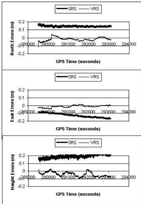
Fig. 5. OSLs station kinematic position accuracy by using the SRS and the VRS methods
