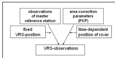
Fig. 1. Generation of the S-VRS data (adapted from [22])
