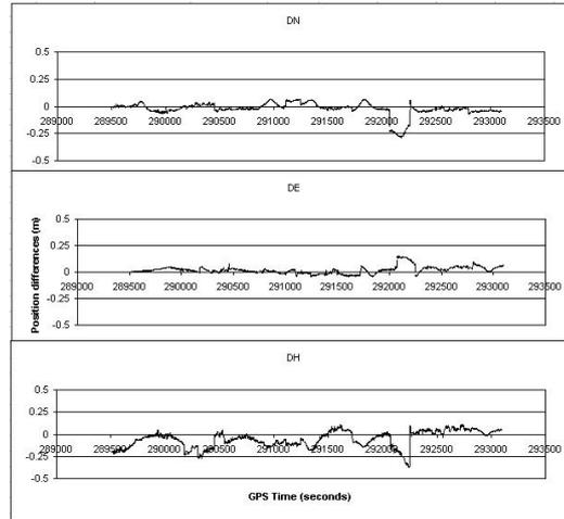
Fig. 8a. Norway airborne GPS kinematic position accuracy by using the S-VRS method
