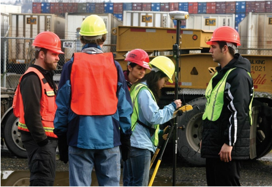
Engineering/survey students with Seattle University learn about the effects of multi-path on RTN observations. The port container facility provides ample multi-path hazards for these lessons.
